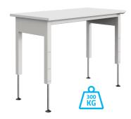
The end cheeks are made of folded sheet steel in L-shape, cross-section 195x40. The ladders are connected via 2 cross-members and 1 base sheet: all 3 in the upper section under the worktoD. The legs and ladders tubes dare fitted with plastic end caps with screw jacks for levelling purposes.
