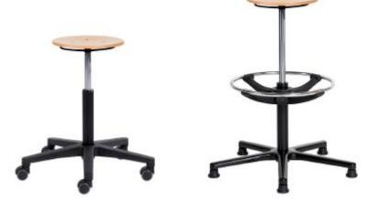
5-star base, in cast aluminum with black powder coating (epoxy) or polyamid reinforced by nylon. Optimization of the stool stability according to its height by diameter adjustment. Castors for hard floor or sliders. Optional footrest for the high version. In compliance with NFD65 761.
